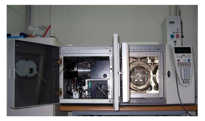
The insides of the GC-MS, with the column of the gas chromatograph in the oven on the right.
